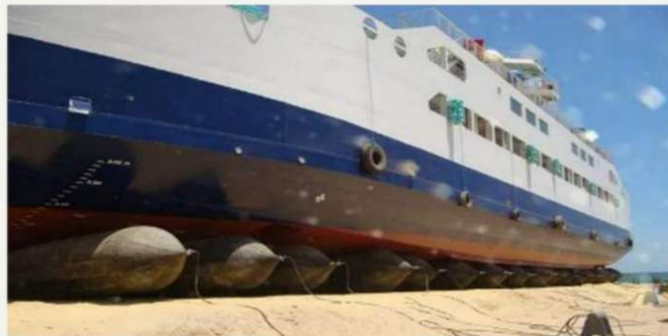
Air bag launch system up to 3500 tons
