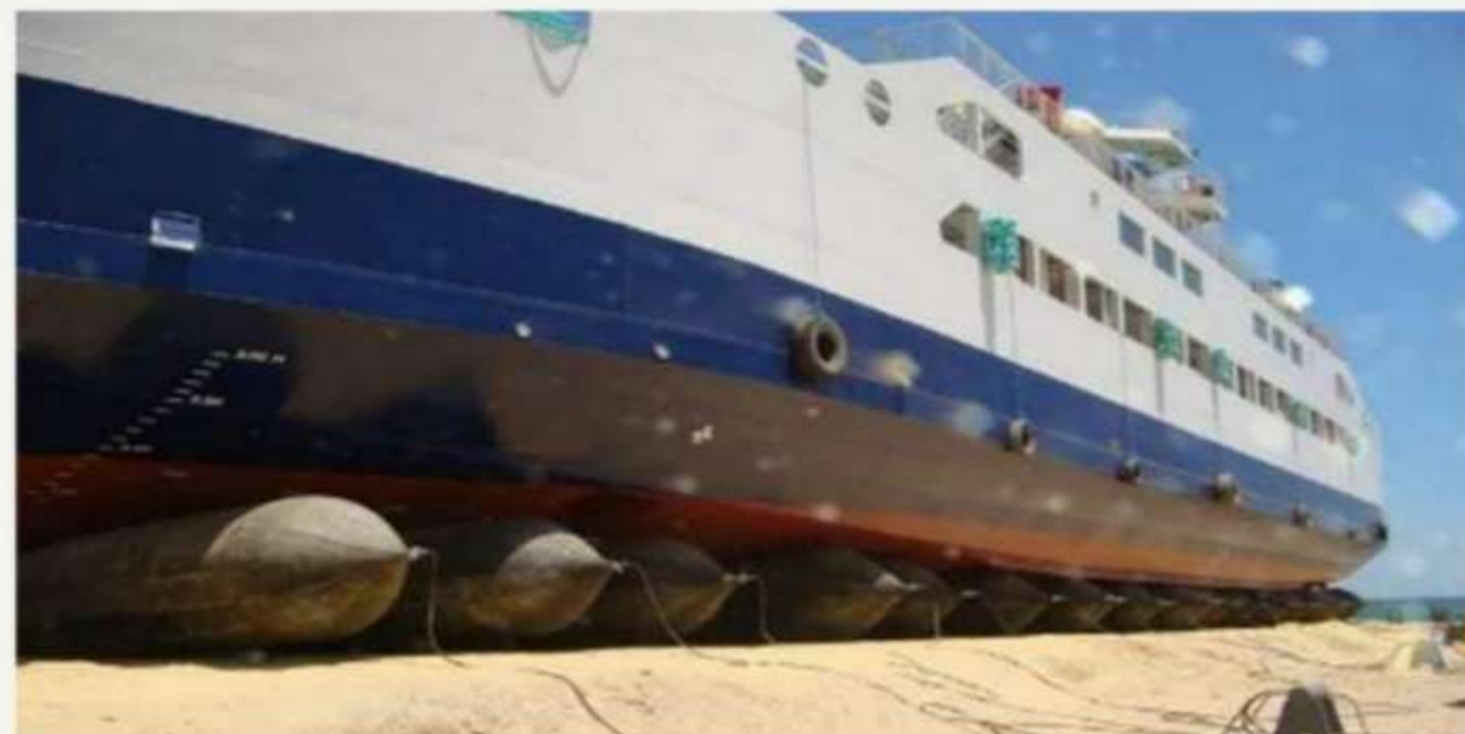
Air bag launch system up to 3500 tons
